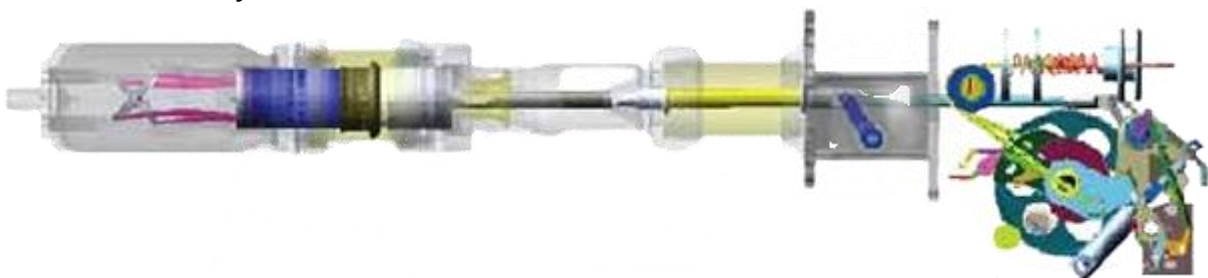
Simulation analysis of mechanism motion process of circuit breaker
