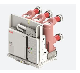
ABB offers its new vacuum generator circuit breakers at 15 kV, 4000 A, 63 kA in accordance to the new Dual Logo IEEE/IEC 62271-37-013 standard to satisfy your business needs in power generation applications.
