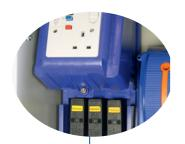
The instrument panel consolidates the digital multi meter, auxiliary fuses and generator synchronisation sockets in one compact panel.
