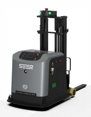
Laser SLAM Counterbalanced Autonomous Forklift
