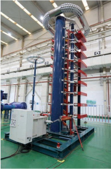
— Lightning Impulse Test Device
