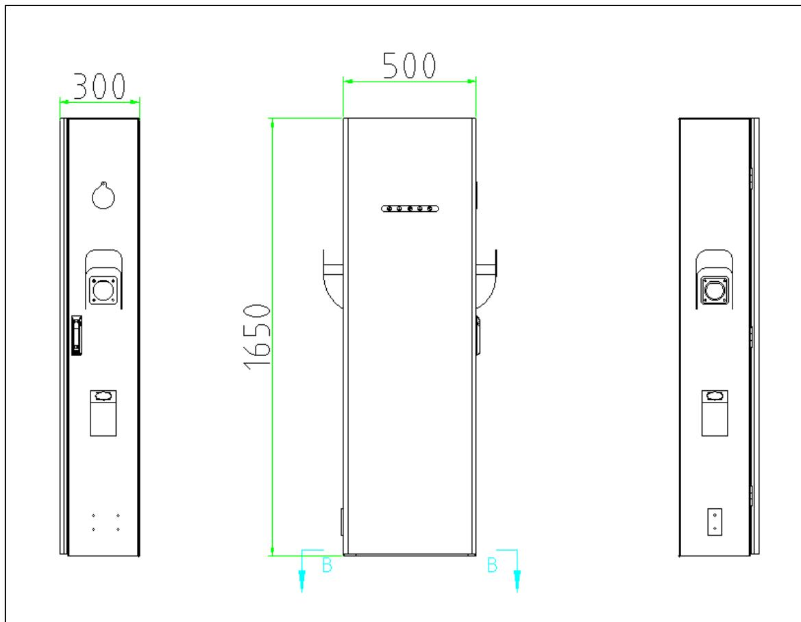
Use 4 x M10\*120 stainless steel expansion screws to secure the charging post. As shown in the figure below. After installing the stake, shake the cabinet from different directions and you should not feel any obvious looseness or shaking.
