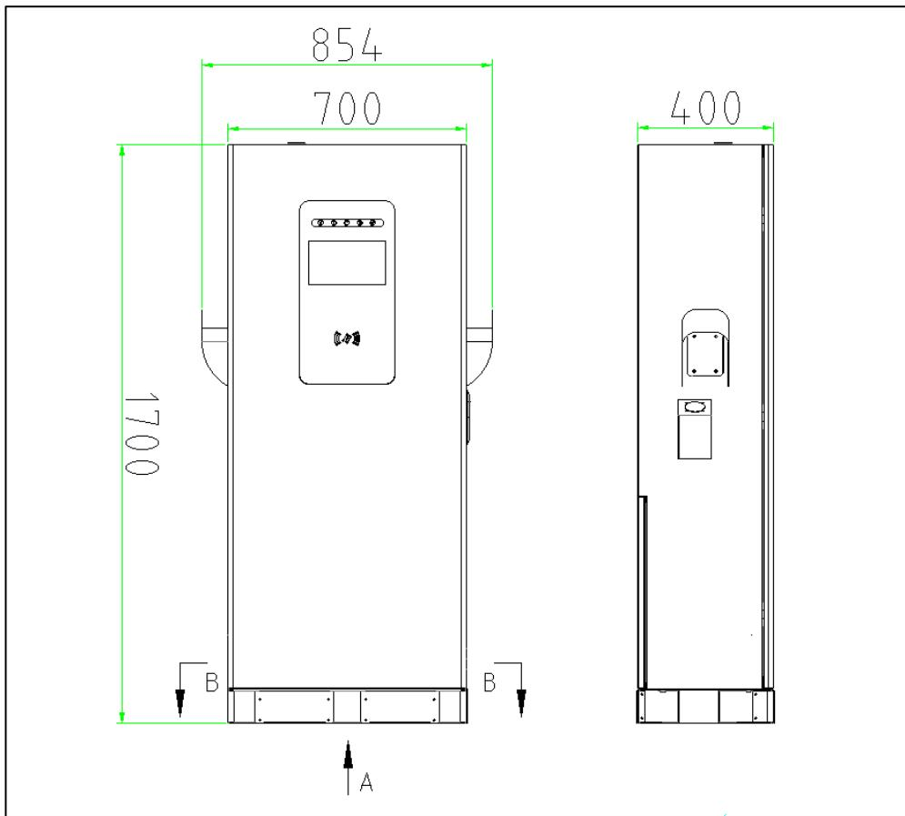
Use 4 x M10\*120 stainless steel expansion screws to secure the charging post. As shown in the figure below. After installing the stake, shake the cabinet from different directions and you should not feel any obvious looseness or shaking.
