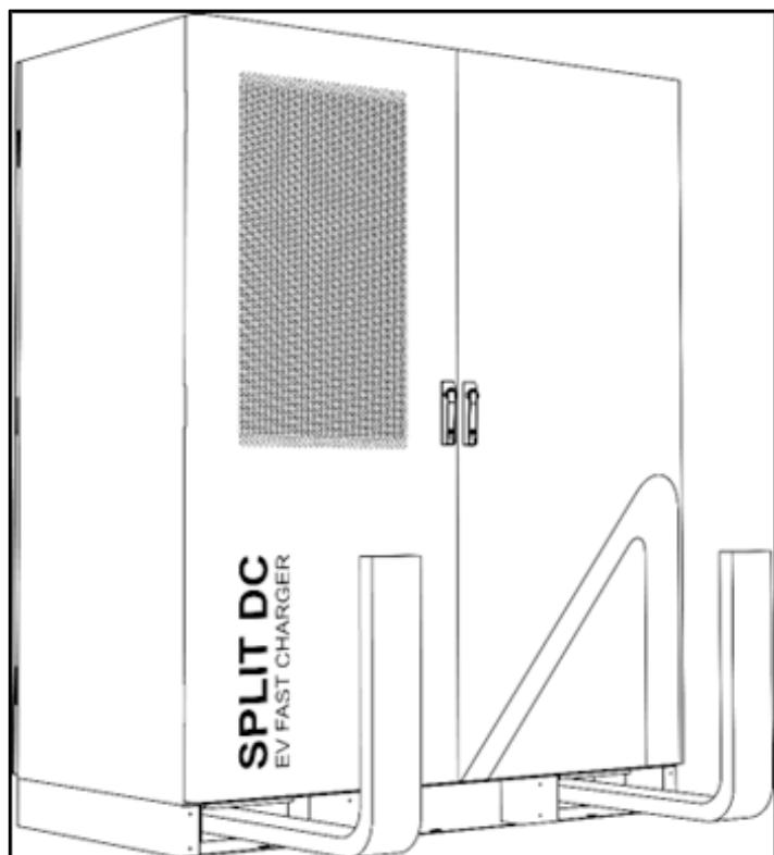
7、Use 6 M12\*120 stainless steel expansion screws to fix the charging pile. As shown in the figure below. After the pile is installed, shake the cabinet from different directions, you should not feel any obvious loosening and shaking.
